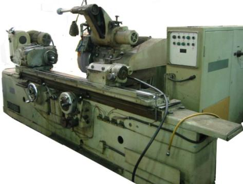
A photograph of a Schaudt ID/OD Grinder. It is a long, horizontal machine with various mechanical components, a worktable, and a control cabinet at the end.                       | 1   | <p><b>Schaudt</b></p> <p><b>ID/OD Grinder</b></p> <ul style="list-style-type: none"><li>• Capacity 14" x 60"</li></ul>                 |
