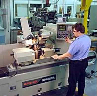
A photograph of a Shigiy Seki GPS-40 ID/OD CNC Grinder. A worker is standing next to the machine, operating it. The machine has a control panel with multiple displays and buttons. | 1   | <p><b>Shigiy Seki GPS-40</b></p> <p><b>ID/OD CNC Grinder</b></p> <ul style="list-style-type: none"><li>• Capacity: 16" x 36"</li></ul> |
